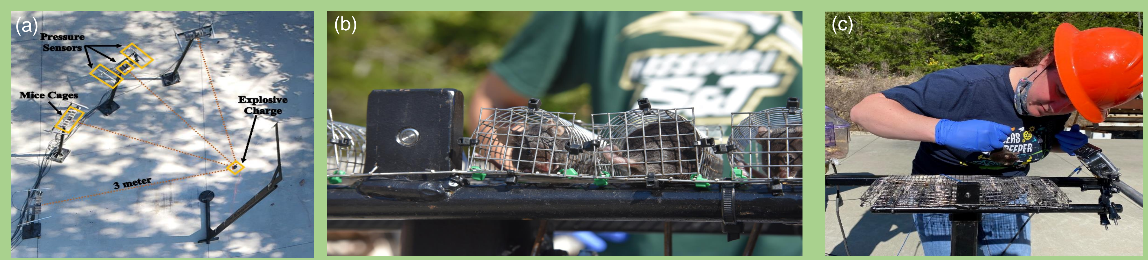
Fig 3. Missouri Blast Model. (a) four stands, each with six mice cages, two pencil probe pressure sensors to measure the static pressure of the blast wave, and one flush mount pressure sensor to measure the reflected pressure of the incident wave. All stands are secured 3 meters from the explosive charge and hold the mice 1 meter off the ground. The explosive charge consists of 350g of C4 hanging 1 meter above the ground. (b) mice in cages. (c) Jenn putting mice into cages
