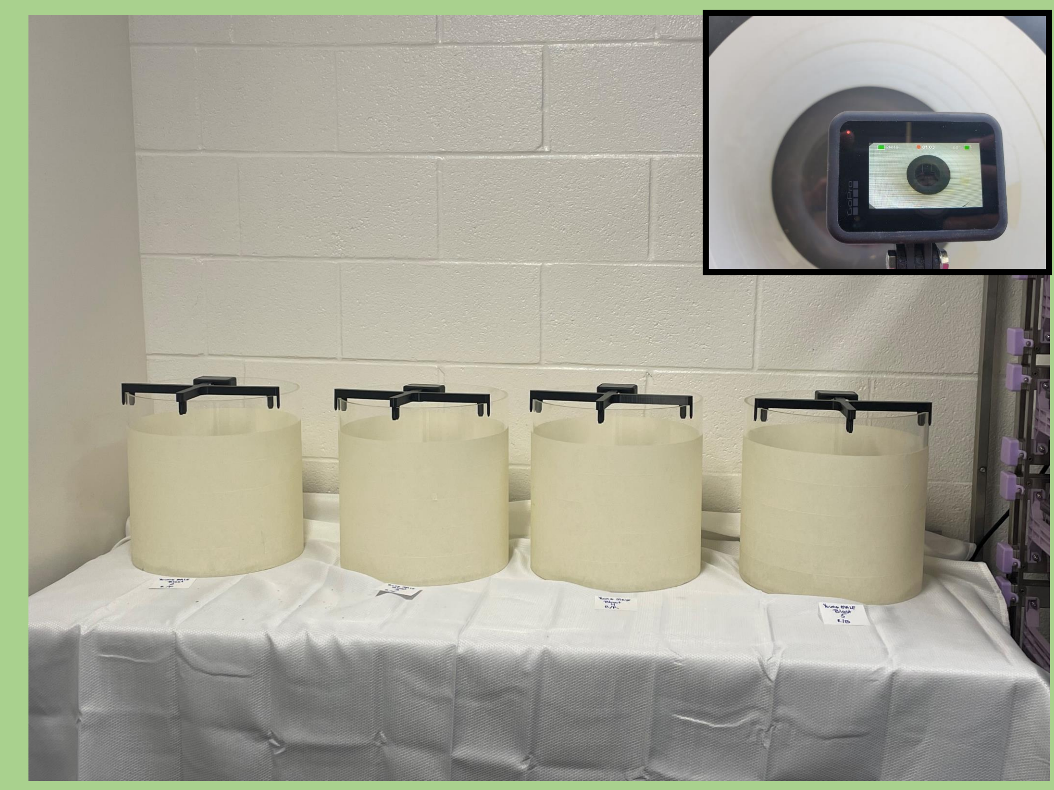
Fig 5. Custom built chambers using GoPro mounts on top for video recording mice. Insert: GoPro camera set-up looking into chambers.
